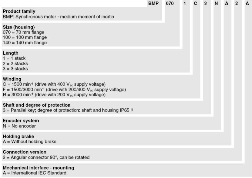
1) In the case of mounting position IM V3 (drive shaft vertical, shaft end up), the motor only has degree of protection IP50.
