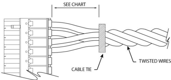
In case of twisted wires, fix the twist with a cable tie and let the cables free for the minimum distance you can see in the table.
