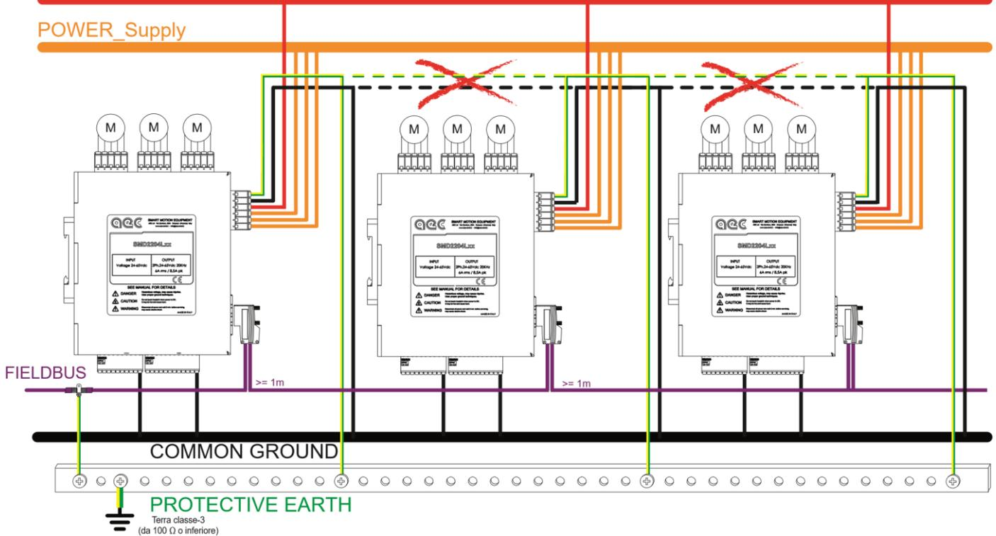
**CAUTION !!!** A wrong positioning, connection, shielding or grounding of the drives or devices connected to the drives, may cause electromagnetic disturbances. The presence of EMC disturbances in electric cabinets may cause malfunctioning of high speed inputs and communication lines.
