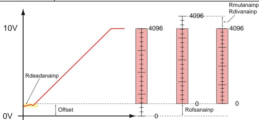
As shown above, it is possible: to create a dead band (yellow zone) in order to eliminate disturbances of the reference in proximity of the minimum value; to shift the analog register in order to let the 0 value coincide with the reference minimum value (Offset); to compress or to expand the scale in order to let the value 4096 (full scale) coincide with the maximum reference value (Rmulanainp and Rdivanainp). In this case, the value of the analog register will be:
