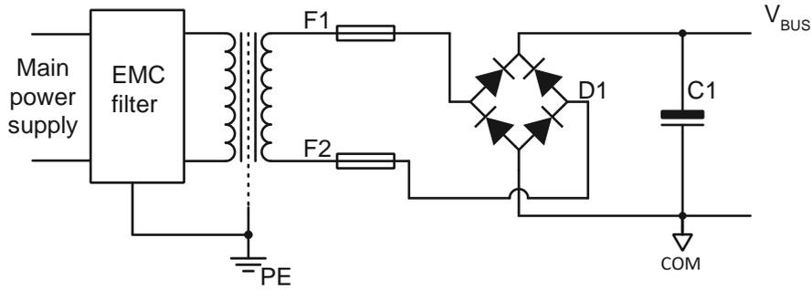
In order to reduce the influence of EMI disturbances, it is recommended the use of our AC/DC converters with intergrated filters AL1120 or AL2620, or as an alternative, of a specific network filter (like CORCOM 10AYO1 in case of three-phase supply, or CORCOM 10VT1 in case of single-phase supply).
