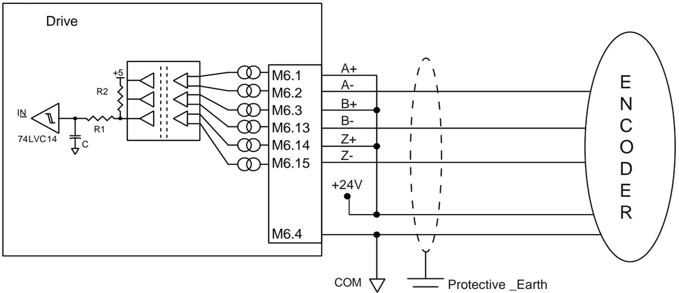
**Place the motor cable at a distance of at least 300 mm from signal cables (encoder, analogic, fast inputs).
