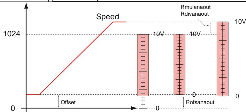
As shown above, it is possible to act on the offset register and on the multiplication and division constant in order to shift the analog register, with the purpose to let the value 0 coincide to the minimum reference value (Offset) and to compress or dilate the scale with the purpose to let the value 1024 coincide to the maximum reference value (Rmulanaout and Rdivanaout).
