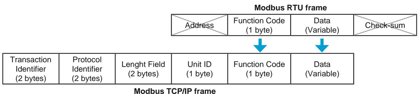
The Modbus commands and user data are themselves encapsulated into the data container of a TCP/IP telegram without being modified in any way.
