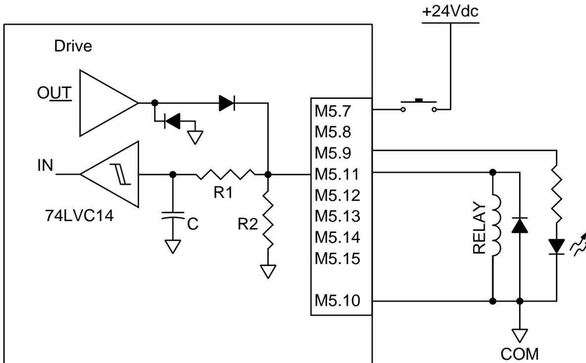
**Caution!!! In case you need to drive inductive loads (like relays, electro-valves, etc.) connect a flyback diode (1A @1000V) in parallel to the load.**
