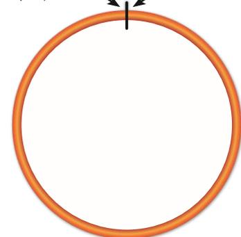
Moving the motor forward, at the exceeding of the upper limit, the quota returns to 0 and continues to increment. In the opposite case, with the motor moving backward, at the exceeding of the lower limit, the quota is imposed at the value of the module quota, continuing to decrement.
