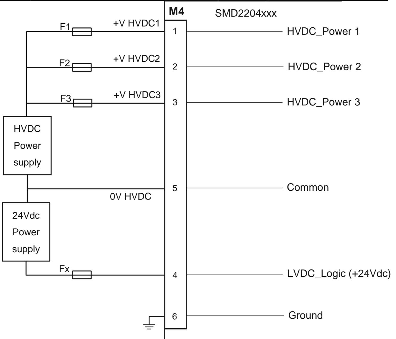
The configuration of the input circuit independently supplies the control stage with respect to the power stage. This solution allows to keep active the indexer (axis controller) in an absolutely safe condition.
