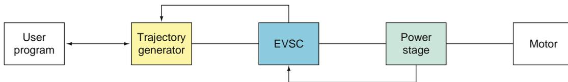
Diagram of the open loop chain of control
