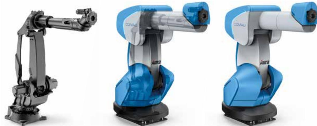
With AURA we transform a standard Comau Hollow Wrist robot into a collaborative solution.
