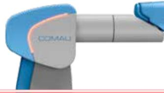
**No LED:** high speed mode, not collaborative (laser scanner installed)
